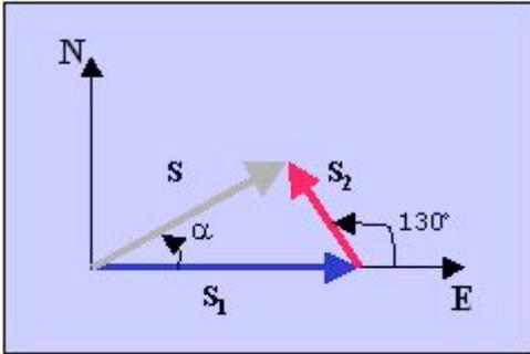
$$S_{1x} = 20\text{km} \quad S_{2x} = S_2 \cos \alpha_2 = 10 \cdot \cos 130^\circ = -6,4\text{km}$$
