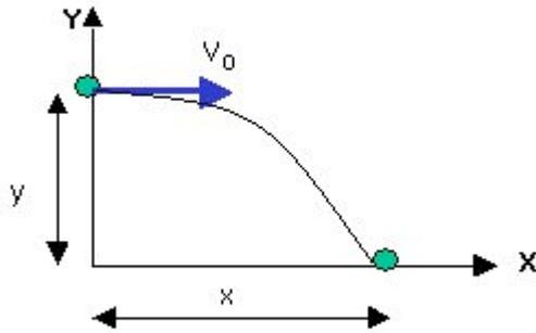
$$y = \frac{g}{2V_0^2} x^2 \Rightarrow 2yV_0^2 = gx^2 \Rightarrow V_0^2 = \frac{gx^2}{2y} \Rightarrow V_0 = \sqrt{\frac{gx^2}{2y}} = \sqrt{\frac{9,8 \cdot 2000^2}{2 \cdot 49}} = 632 \text{ m/s}$$
